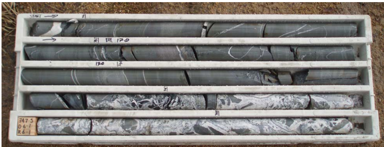
Drill core showing sharp transition between metasedimentary host rock and colloform banded quartz-sulphide vein breccia; PMD001 – 743.85 – 748.38m Porters Mount Prospect – July 2008 ©
