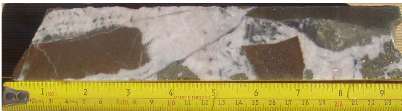
Drill core sample showing angular fragments of pink micromonzonite and pyrite aggregates entrained in vein breccia; PMD001 – 755m; Porters Mount Prospect – July 2008 ©
