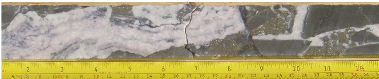
Drill core as above after sampling showing colloform banding in close up; PMD001; Porters Mount Prospect – July 2008 ©
